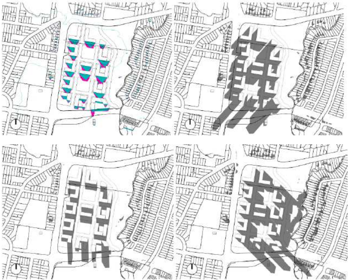
Figure 12: Overshadowing Diagrams during the Winter Solstice L-R: Coloured areas which receive less than 2 hours sunlight; June 21 9am, 12pm & 3pm.
